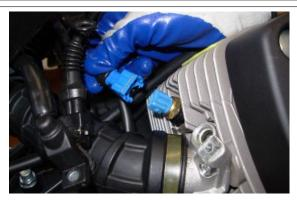
• Connect and secure the injectors
