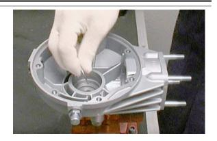
Fit the sealing ring on the housing using the suitable punch (19926000).
