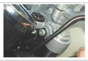
Undo the lower sealing screw.
