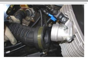
Tighten the clamps, checking correct positioning
