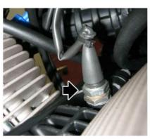
Detach the sensor connector and check the purple cable is ground insulated: if there is
