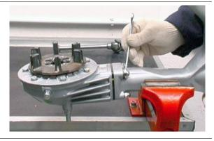
• Slide off the gearcase together with the swingarm.
