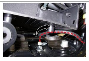
• Connect the speed sensor and rear stop
