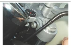
• Unscrew and remove the central nut.
