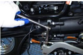
Insert the screws with the relative retainer nuts and washers of the cradles to the frame
