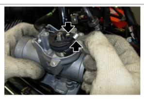
Correctly position the guides and tighten the nuts, checking correct operation of the throttle grip
