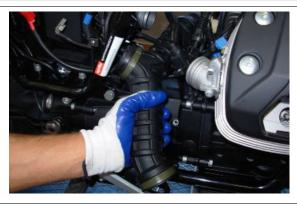
Disconnect the oil pressure bulb connector
