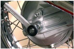
• Loosen the wheel pin locking screw.
