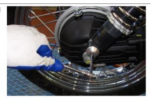
Remove the side pins, taking care to recover the nuts
