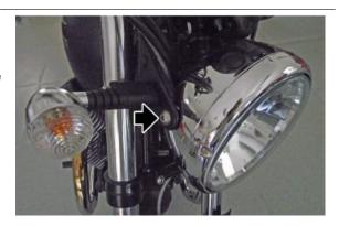
Working from both sides, disconnect the two connectors.
