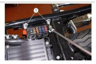
Remove the brake pump unscrewing the two fixing screws.
