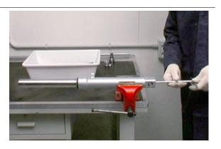
Remove the dust scraper using a screwdriver as a lever.
