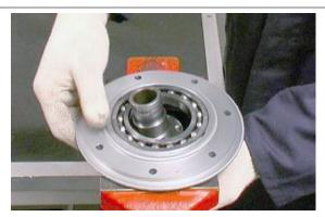
• Remove the sealing ring.
