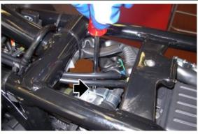
Install the sleeve, taking care that they are inserted correctly
