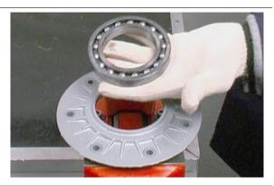
Remove the external ring of the needle bearing from the housing using the suitable extractor (19927500).
