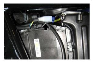
Side Stand Down: open circuit (infinite resistance)
