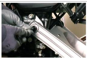
Screw in the lock nuts on the pins, locking them thoroughly.
