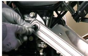
Remove the shimming washer between the swingarm right arm and the gearbox.
