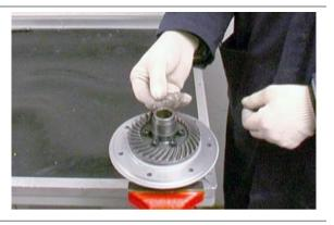
Fit the braking disc on the drilled bolt by locking the screws with the washers using a torque wrench.
