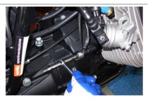
Disconnect the clutch cable from the lever
