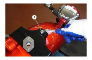
Remove the front screws (2) that secure the mudguard to the frame, taking care to recover the nuts
