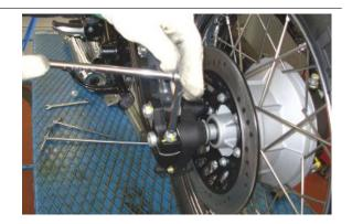
Remove the wheel pin and collect the spacer.
