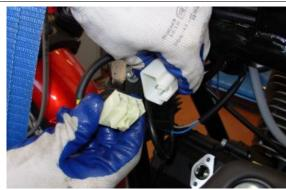
• Connect the spark plug tubes
