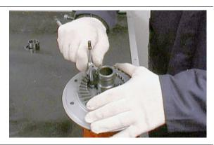
Remove the conical crown.
