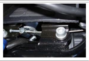
• Connect the clutch cable to the lever
