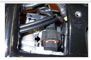
Install the MIU G3 control unit connector support bracket
