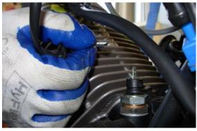
Remove the fixing screw of the engine ground wires
