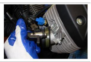
Disconnect the engine temperature sensor connector
