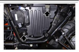
Secure the filter box to the frame
