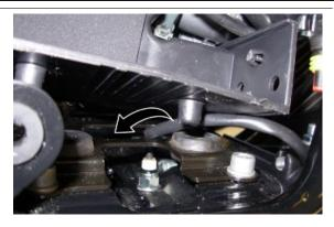
After removing the clamp, disconnect the speed sensor and rear stop
