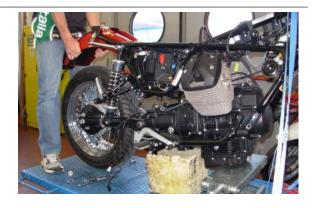
Insert the central pin from the right side of the motorcycle, place the washer and the nut from the opposite side
