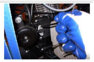
• Disconnect the alternator connector
