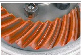
Fit the drilled bolt-crown unit cover and their spacers and gaskets on the housing and provisionally tighten the screws.
