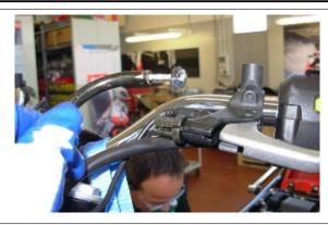
Disconnect the clutch cable from the disengagement lever
