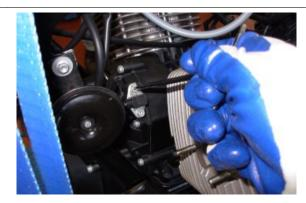
• Connect the alternator connector
