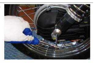
Attach the rear left shock absorber via the appropriate pin with corresponding nut
