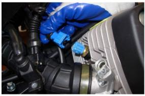
Loosen the clamps securing the sleeve and remove it
