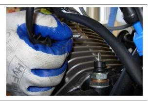
• Attach the engine ground leads
