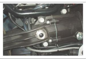
Loosen the pins so that the oscillating swingarm can be removed from the gearbox.
