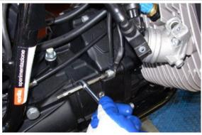
Connect the engine temperature sensor connector
