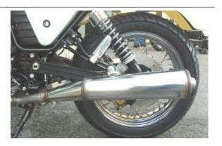
Remove the rear calliper, releasing the brake pipe from the retainers on the swingarm.
