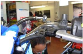
Install the sleeve, paying attention to the correct positioning of the clamps before tightening them
