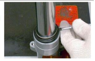
• Slide the dust scraper off and upwards.
