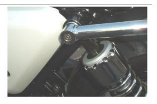
• Undo and remove the lower screw.
