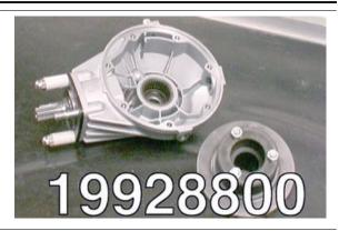
Insert the tool on the bearing cage in the housing.
