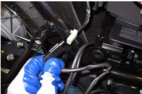
Connect the clutch cable to the trip lever
