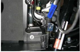
Unscrew and remove the lambda probes.
