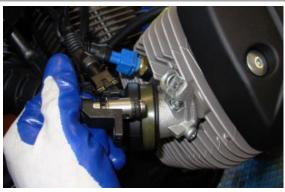
Install the timing sensor with its seal
