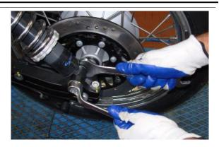
Remove the screw fixing the right-hand rear right shock absorber and pull it from the pin on the drive shaft
