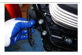
Remove the screws fixing the cradle, making sure to recover the nuts and washers
