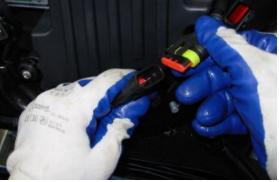
Disconnect the right Lambda probe connector and slide the cabling from the cable grommet
