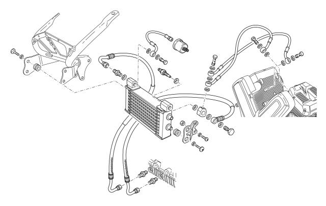
Diagram of the blow-by and piston cooling circuit
