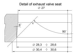
Detail of exhaust valve seat
