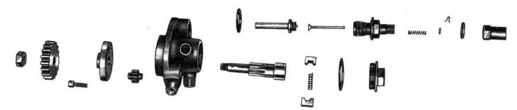
Figure 25- Oil pump dismantled: one notices the sequence of dismantlement.
