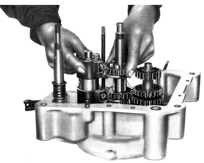
Figure 22- How you must assemble the gear change into the left half of the crankcase.
