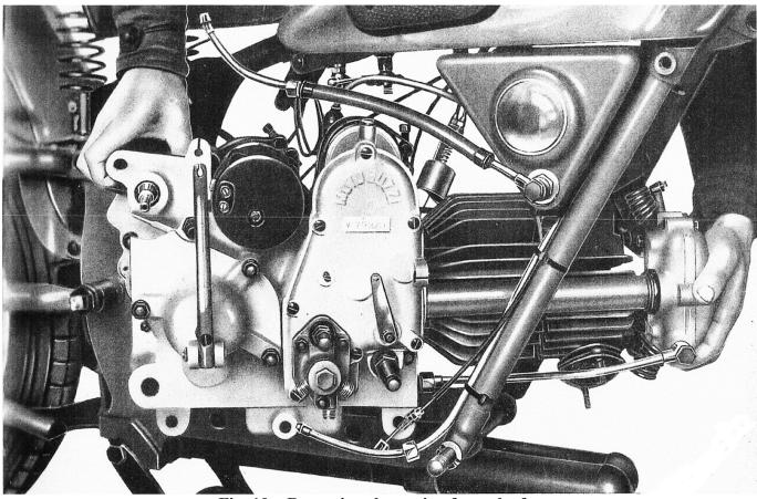
Fig. 10 – Removing the engine from the frame.
