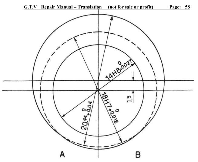
Figure 26- Diagram center of the vanes on the oil pump.
