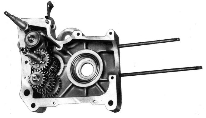
Remove the crankshaft unit, complete with connecting rod, by suspending the right crankcase half by hand and beating the crankshaft with a wooden mallet from the exterior toward the interior.
