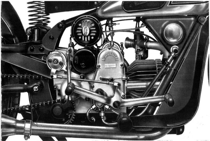
Fig.7 – Engine unit mounted in frame.
