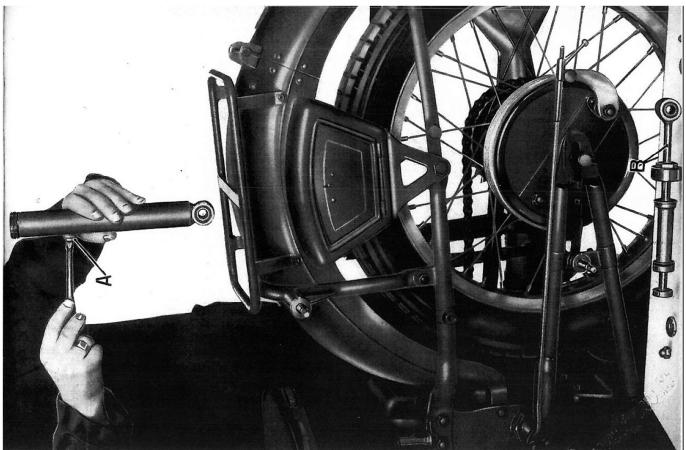
Figure 36- Verification of the liquid in the dampers.
