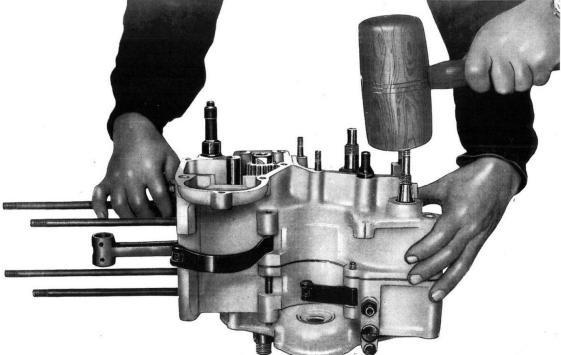
Fig.14 – Opening the crankcase.
