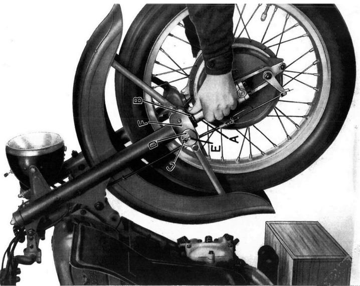
Figure 35- Adjustment of the telescopic fork.
