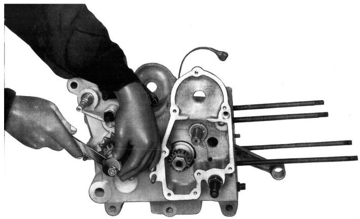
Fig.12 – Disassembling the clutch rod.
