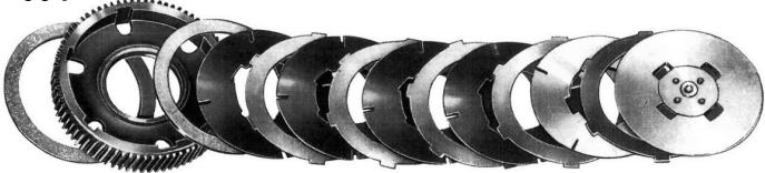
Figure 21- Dismantled clutch (notice the order of assemblage of the varied pieces).
