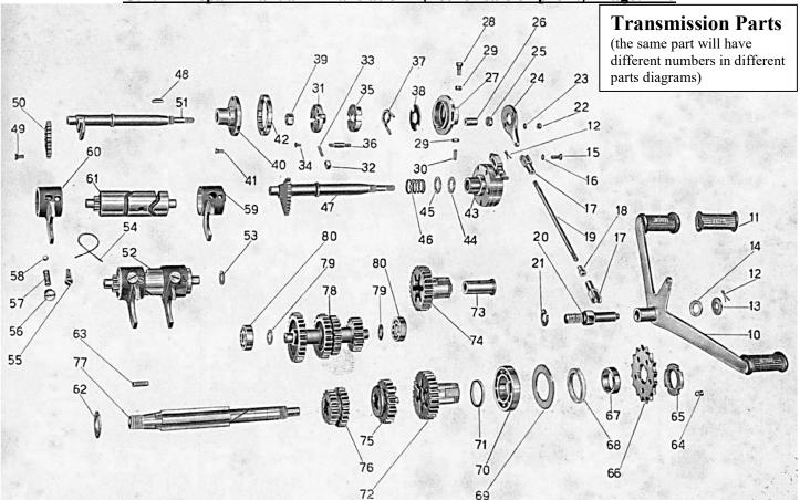
Assemble the mainshaft by aligning the keyway and inserting the tapered end into the taper of the clutch fixed body. Don't forget the spacer ring which is assembled with the flat side toward the bearing [#62 in parts diagram – left side bearing not shown. photo B].
