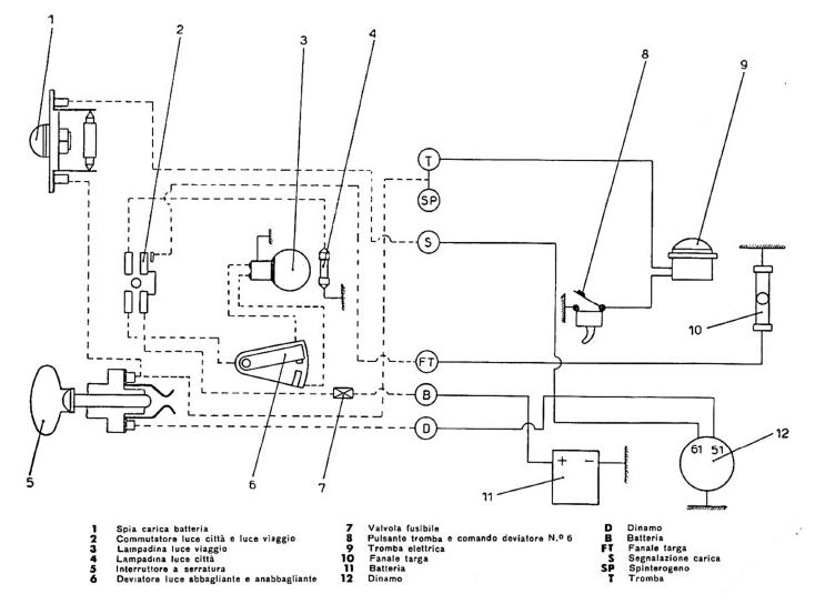
Figure 27- Diagram of the connection of the electric installation.
