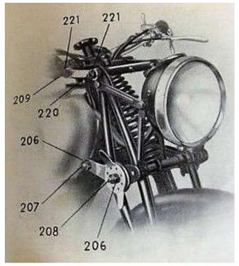
With the left link removed the respective nut is screwed back onto the left end of pin 207, bottoming it, and the two counter-nuts 206 are screwed onto the left end of pin 208, tightening them against each other. This makes it possible, by turning the pins 207 and 208 counterclockwise (from the left side of the machine) to extract the pivot pins completely from the right-hand lower link.
