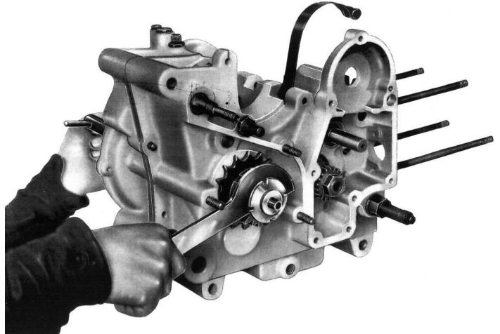
Fig.13 – Removing the toothed sleeve (ratchet) for the kickstarter. [Flywheel lockring tool is the same size.]
