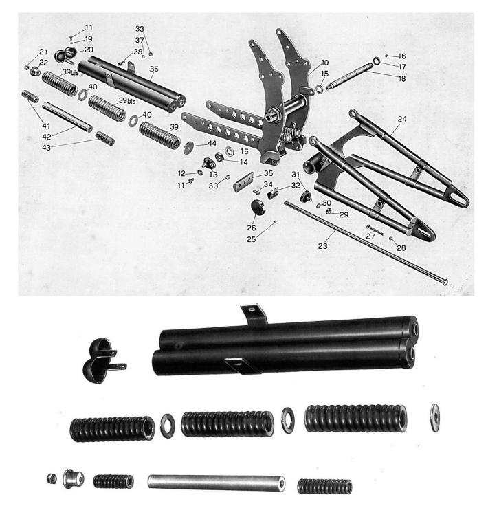
Figure 31- Springs and carrier tubes: notice the group is removed from the suspension.
