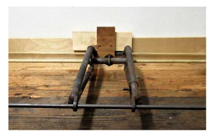
the long edge of the square against the pivot eyes and compare the alignment to the ends of the straight rods. Side links are straight with both ends of the link in the same plane (in other words the thickness of the bronze washers should be the same at both ends of the link.). Upper links are 8 mm thick at pivot pin eyes. Lower links are 11 mm thick at pivot pin eyes.
