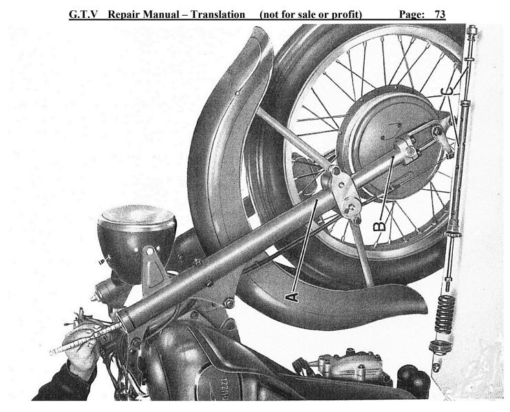
Figure 34- Verification of the liquid in the telescopic fork.
