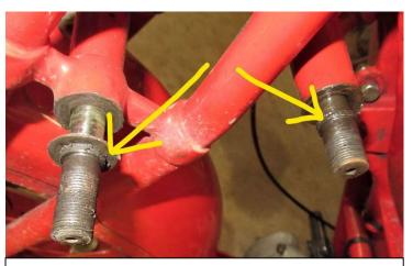
Left link removed. Arrows mark shoulders that prevent pivot pins from being pulled through to the right.
