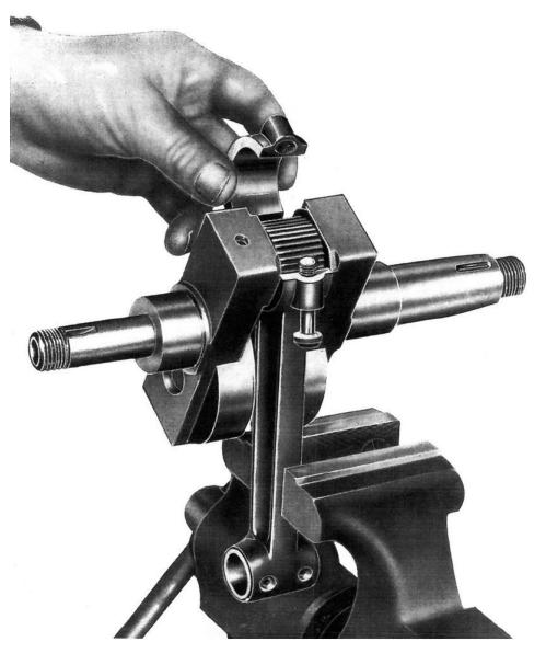
Fig. 20 - How to assemble the connecting rod and the needles on the crankshaft.
