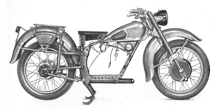
Figure 30- Frame ready for dismantlement.
