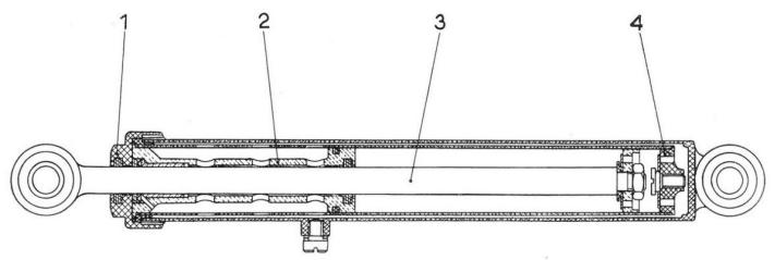
Figure 33- Internals of the rear dampers.
