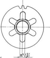
After pressed in place, lathe roughly to 18,5 +/- 0.02 then ream precisely to 18,58 +/- 0.01.
