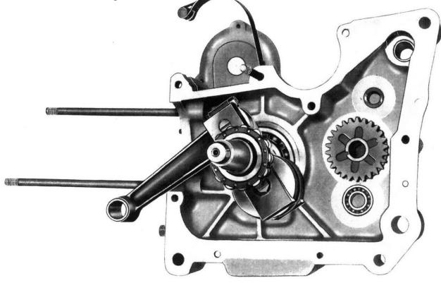
On the left crankcase half (flywheel side) will remain mounted the shift control shaft with toothed arc, the transmission gear clusters and the shift control cylinder with the relative shift forks – Fig.16.
