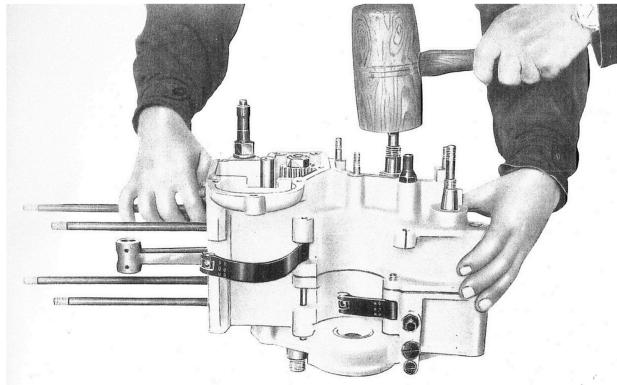
Fig.15 – Opening the crankcase.
