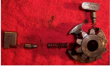
In summary, this is the way you want the notched pawl to sit within the shift drum and its covering camplate. The notch is UP and IN. Mirror the position for the one on the opposite side.
