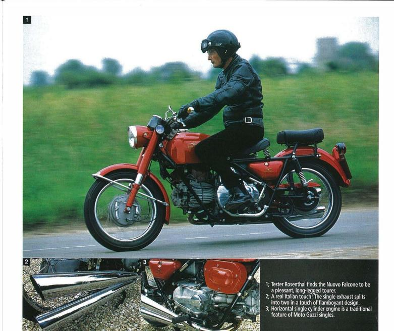
before we hit the road. Despite being a heavy single, the Nuovo Falcone carries its weight well with a low centre of gravity thanks to the low slung horizontal engine, which combined with its narrow build, would make manoeuvring around the workshop or even into the garden shed relatively easy. Likewise, hoisting it onto its centre stand needs effort but not that much. It's a refreshing change, from some of its top heavy Oriental rivals!
