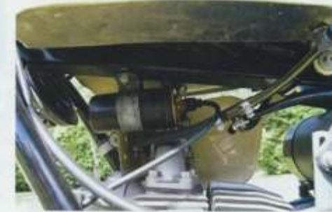
Under the beige tank live the carb, the coil and the great big starter motor / generator. There is plenty of room...
