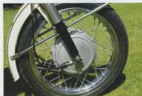
On the opposite side of the front wheel to the brakeplate is the speedo drive. Almost modern. As is the front fork, which works very well indeed
