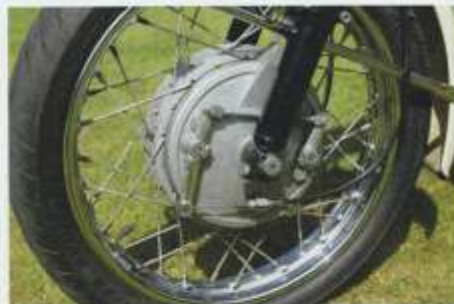
One excellent twin leading-shoe brake. It is indeed excellent, and suits the bike very well indeed
