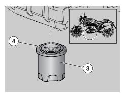
◆ Unscrew oil filter (3) and remove it.
