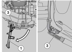
The side stand (1) is equipped with a safety switch (3) that inhibits ignition or stops the engine whenever a gear is engaged while the side stand (1) is down.
