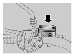
The clutch reservoir is located on the left handlebar, close to the clutch lever fitting.
