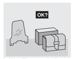
Avoid installing accessories that cover horns or lights or that could impair their functions, limit the suspension stroke and steering angle, hamper operation of the controls and reduce the distance from the ground and the angle of inclination in turns.
