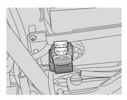
First check the secondary fuses, then the main fuses.
