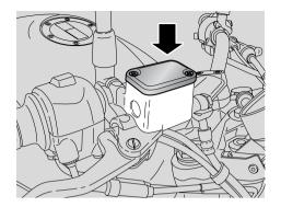
The front brake fluid reservoir is located on the right handlebar, near the front brake lever connection.
