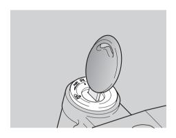
Before replacing a bulb, set the ignition switch to "1" and wait a few minutes to allow it to cool.
