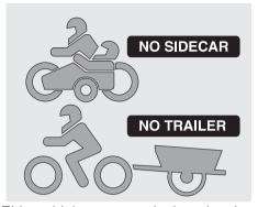
This vehicle was not designed to be equipped with a sidecar or to be used to tow trailers or other vehicles.
