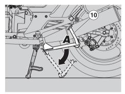
**NOTE** Do not let the side stand touch the ground. Keep the vehicle in vertical position.
