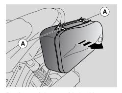
Retainers of the two side buckles must always be secured to bag body fasteners A, no matter if bellow is open or closed.
