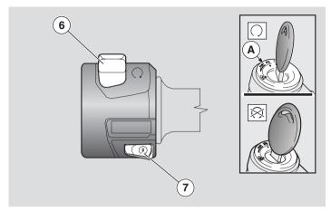
With the switch (6) in the " $\bigcirc$ "(ON) position it is possible to start the engine. The engine can be stopped by moving the switch (6) to the  $\bowtie$  (OFF) position.
