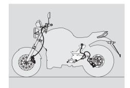
**NOTE** This vehicle is equipped with front and rear disk brakes, with separate hydraulic circuits.
