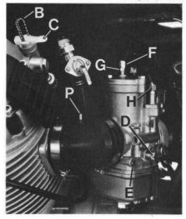
the slides have the same opening. If not, undo locknuts "G" and act on adjusters "F".
