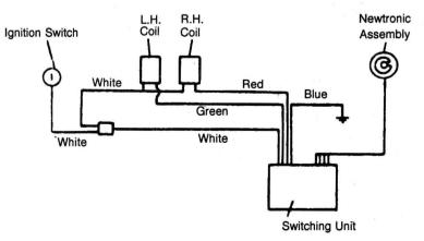
SCHEMATIC WIRING DIAGRAM
