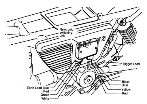
NEWTRONIC SWITCHING UNIT IN L.H. SIDE PANEL
