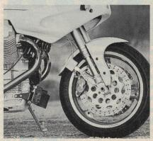
The 40mm inverted WP fork replaces the conventional Marzocchi legs from the carbureted Sport. Those 320mm floating rotors and four-piston Brembo calipers provide brick-wall stopping power, and yes, Luigi, those are cast Marchesini rims.
