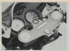
The '97 Sport's control pod is a thing of beauty. Note the machined finish on the triple clamp. The fork is adjustable for compression and rebound damping.
