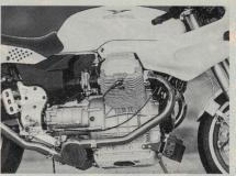
The longitudinally arrayed V-twin remains a most unique mill. An oil cooler has been added for '97, though its lonely post leaves it somewhat vulnerable to road shrapnel.
