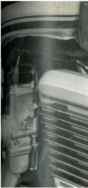
A new, more powerful alternator is keyed to the front end of the crankshaft. Also visible are the two horns, of adequate power for the performance of the bike.
