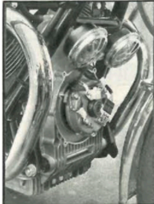
A new, more powerful alternator is keyed to the front end of the crankshaft. Also visible are the two horns, of adequate power for the performance of the bike.
