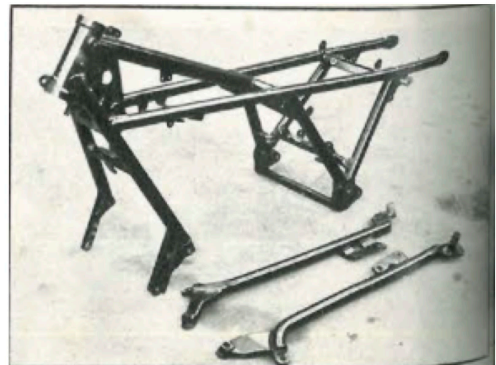
The now famous Moto Guzzi double cradle detachable frame does not require further comments. The view from below shows the extended finning of the sump and the exhaust crossover between the two pipes. A little ahead of the latter you can see the tube coming from the intake box where the crankcase breather gases are routed.
