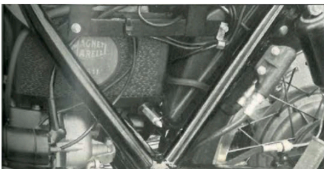
The side panels are mounted elastically with a rather flexible fitting mechanism. Under the right-side one (opposite page) is the foot brake cylinder with numerous components of the electrical system, including the fuse box and the turn signal flasher. Unfortunately, these changes led to the disappearance of the two side toolboxes of the T. The modest supply of tools is therefore placed in a low capacity tray under the saddle without any anti-theft protection. We should add that on the left side, as you can see from the photograph, there would have been enough space for one of the toolboxes to survive. Also on the left, behind the rear tube of the frame, you can see the three-way manifold that connects the master cylinder of the pedal control with a front and rear caliper. For the moment, the use and maintenance booklet of the 850 T is still being distributed with the T3.
