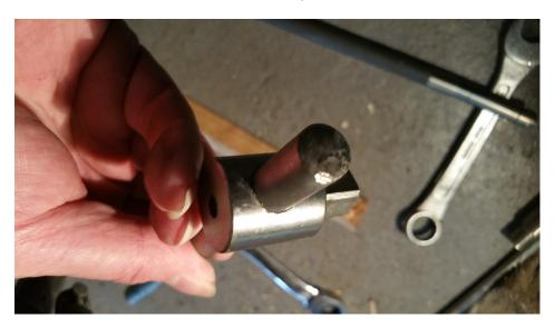
Then I wrapped a piece of cloth around here, clamped some mole grips around and hammered the living daylights out of the moles - nothing
